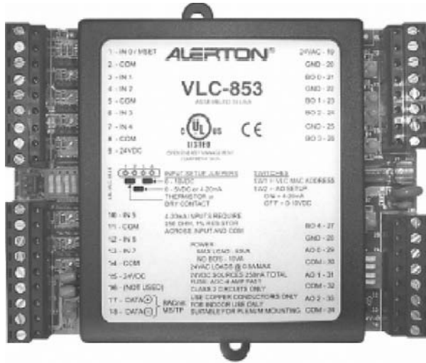
Figure 11-11 Typical Controller Hardware
